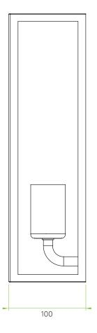
Recess in wall for Terminal Block 60x60x30mm
